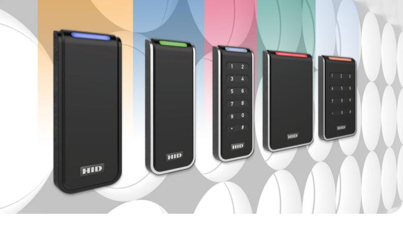
"HID Signo Readers include velocity checking, a patented feature to protect against brute force rapid electronic attacks."
